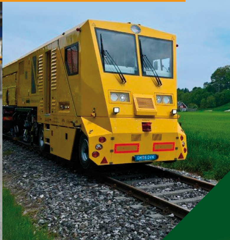
Rail grinding machine now in use
