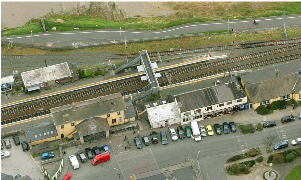
Greystones Station – Platform 1 in the foreground caters for all DART services; platform 2 is accessed by the footbridge and is used for other passing trains. The permanent way sidings are at the top of the photo, along with the signalling interlocking building
