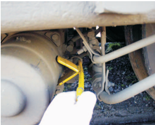
Fig 14 - The parking brake release lever in use.
