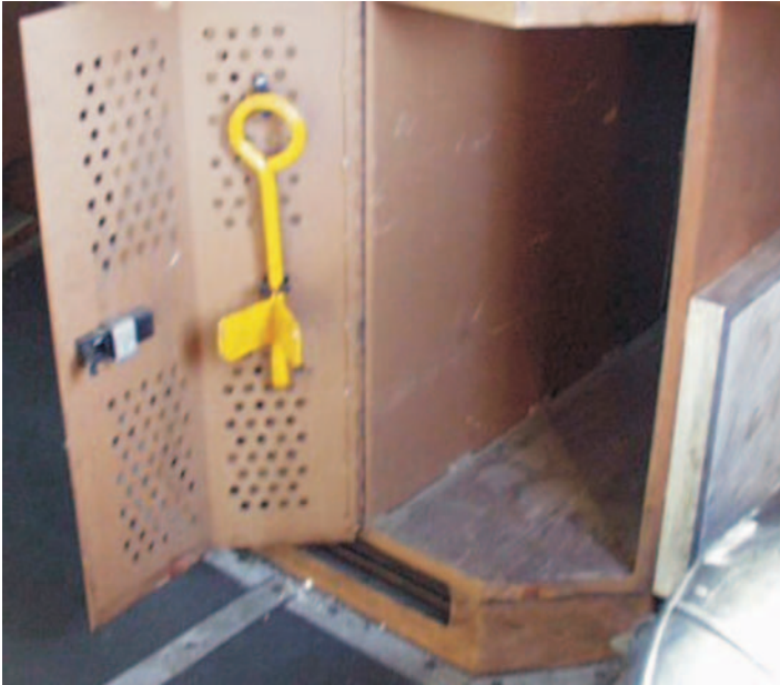
Fig 13 - The location of the parking brake release lever in the driver's cab.
