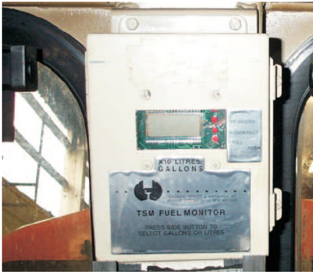
Fig 12 - In-cab fuel gauge located between the two windscreens.
