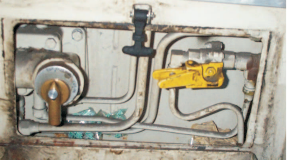
Fig 15 - The MU2 valve to the left of the normal/remote cut-out valve. The cut-out valve is in the normal position.
