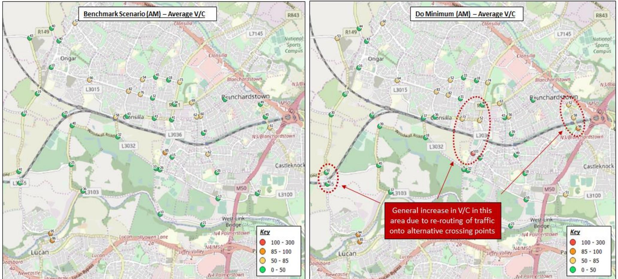
Figure 6.4 AM Average V/C – Do Minimum vs Benchmark Scenario
