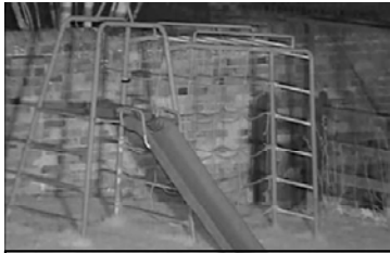
Night scene with IR Lighting at 70 metres
