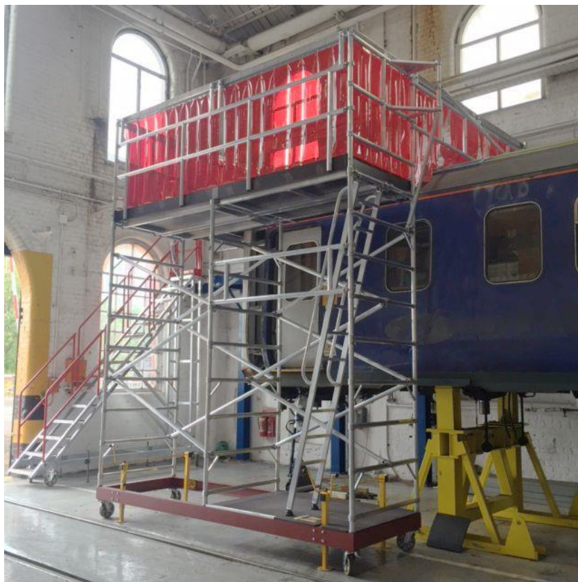
Figure 6-1 Sample "Boxing Ring" vehicle roof access platform
