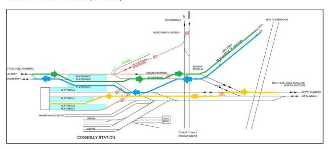
This therefore means that terminating services from either the GSW or Newcomen Lines can access and Depart Platform 7 without conflicting with Northern Line moves. Services can be operated on an arrival and departure pattern from the same lines, or, if it can deliver more services, it could be possible to arrive from one route and depart to the other.
