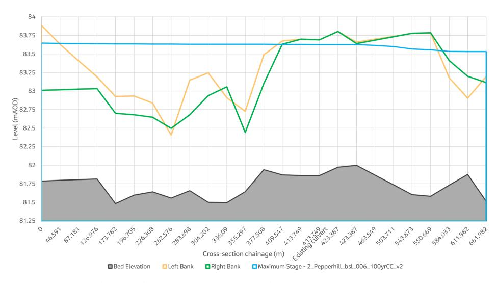
Figure 8: Maximum Water Level profile predicted for a 1 % AEP Event plus Climate Change for the baseline scenario on the Pepperhill Tributary
