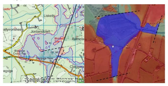
Model boundaries in Inset Figure 1.13 are illustrated in dashed black lines, flood extents illustrated in blue, red shading on right hand side shows higher ground based on LiDAR
