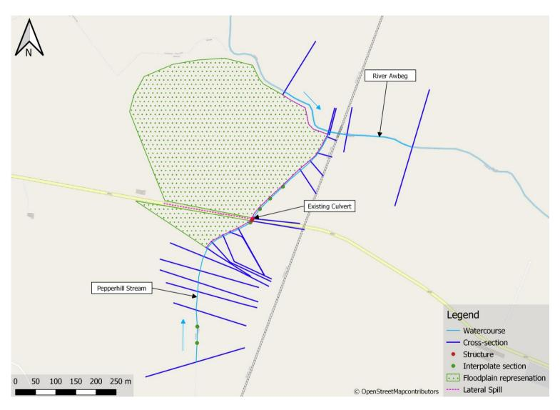
Figure 2. Model schematisation (baseline scenario)
