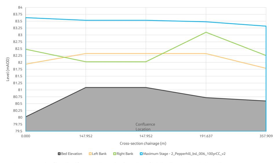
Figure 9: Maximum Water Level profile predicted for a 1 % AEP Event plus Climate Change for the baseline scenario on the River Awbeg
