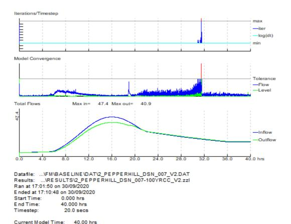
Figure 6: 1D Model Convergence – 1 % AEP Event plus Climate Change (Scheme)
