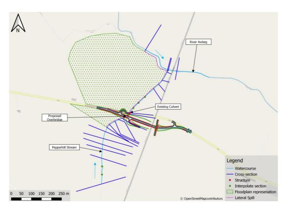
Figure 4: Scheme Scenario (new bridge with box culvert)
