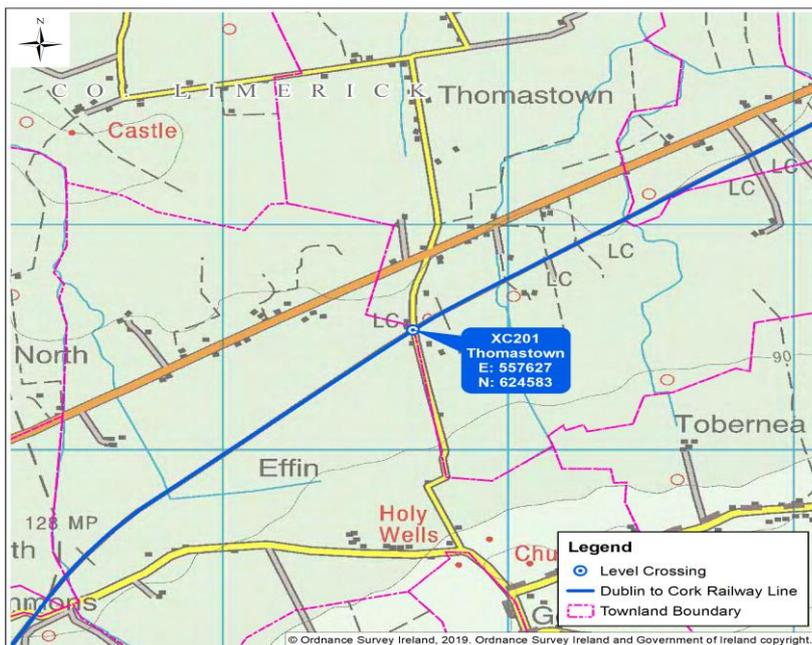
The crossing is manned 07.30hrs-23.30hrs and the gates are normally closed to road traffic, with the gate keeper opening the gates as required. The crossing is closed to road traffic from 23.30hrs until 07.30hrs. Similar to XC187 Fantstown, the length of time that the road user is waiting depends on when they arrive at the gate and if a train has left Limerick Junction or Charleville. The road user has to wait until they pass.
