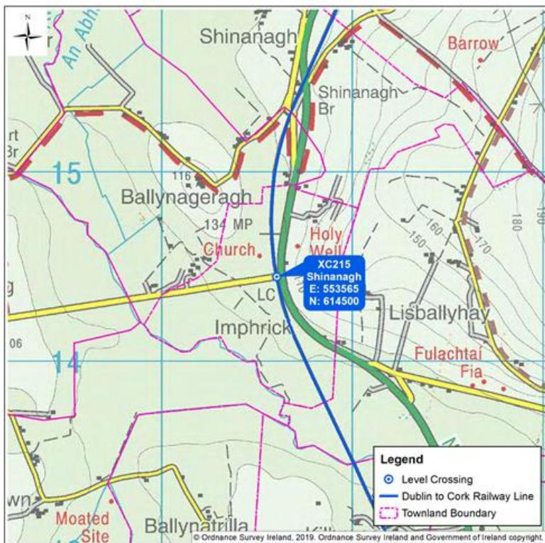
XC215 Shinanagh is designated a ‘CD-Type’ level crossing but it has been operated as a ‘CX-Type’ level crossing for over 25 years and similar to XC212 Ballycoskery is manned on a 24-hour basis. Its operation as a ‘CX-Type’ crossing results in the gates being normally open to road traffic with the gate keeper closing the gates as required for rail traffic.
