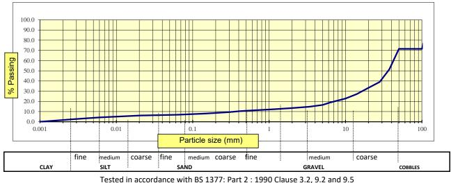
Sedimentation by Hydrometer - Not UKAS
