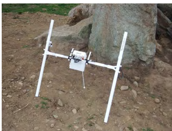
Bartington Grad 601-single axis dual sensor gradiometer.
