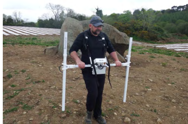
Bartington Grad 601-single axis dual sensor gradiometer.
