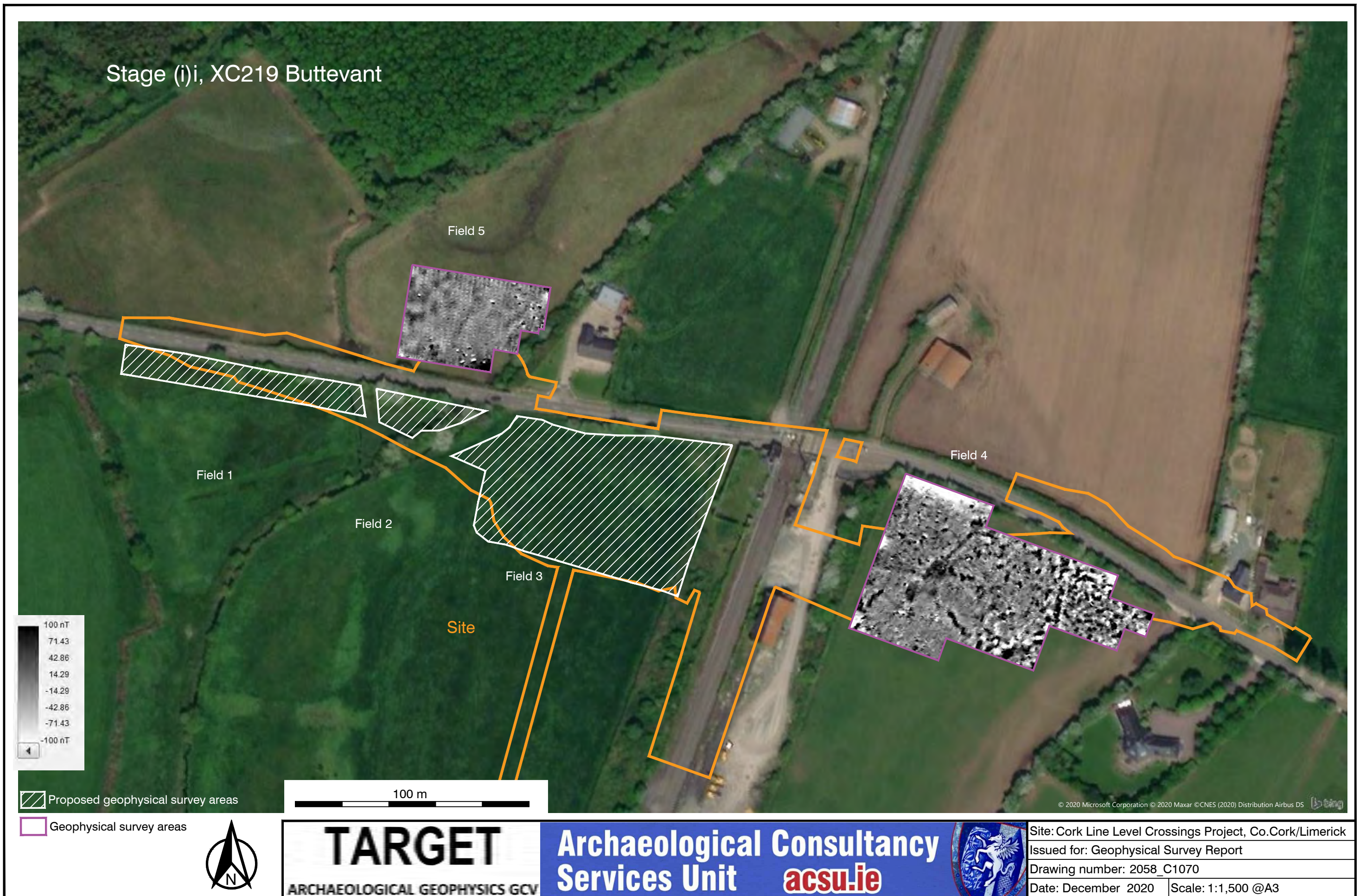
Figure 20: Aerial view of site XC219 Buttevant, showing geophysical survey results (greyscale image)
