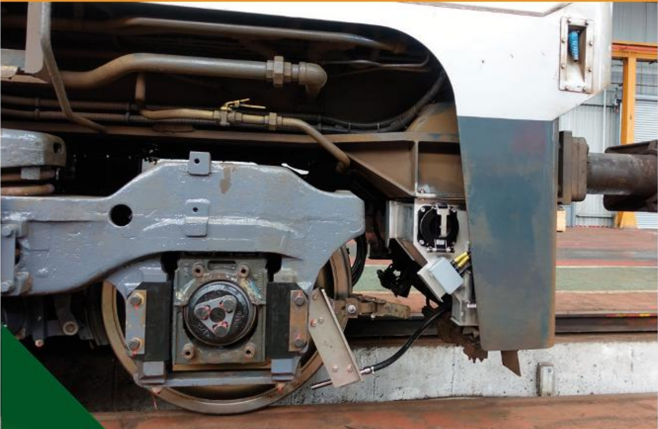
Sandbox behind Cowcatcher supplying sand to nozzle and wheel-rail interface. (Photo K. Marnane)
