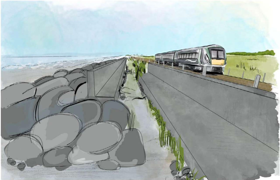
Figure 12: Illustrative view looking South to Newcastle showing the transition from the set back wall to a rock revetment with wave wall
