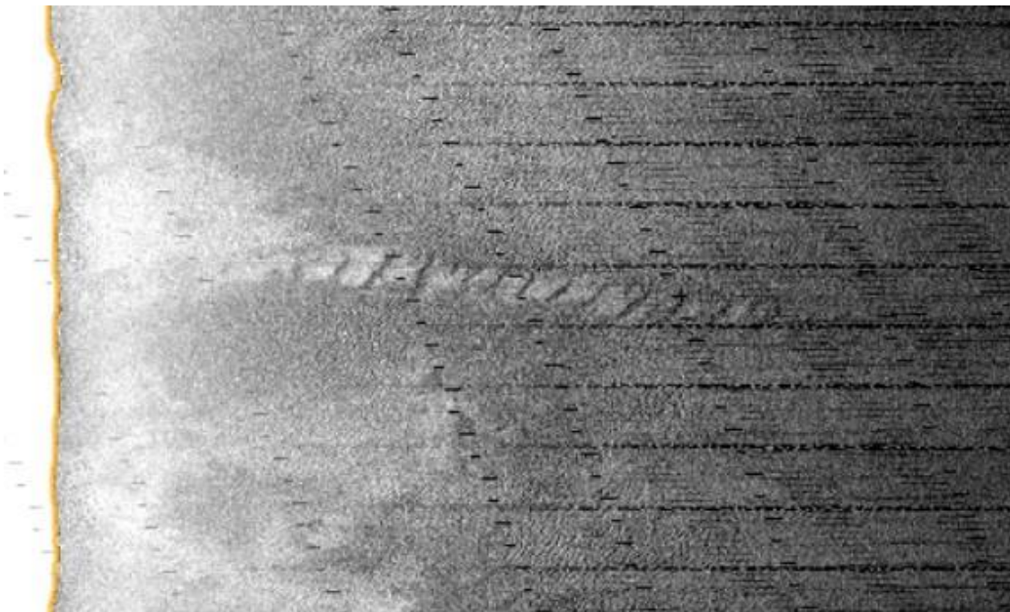
Plate 5: ADCO4. Side scan sonar data trace showing possible line of c. 14 stakes, c. 1m long and c. 1m separations, extending c. 14m in length close inshore in vicinity of and west of
