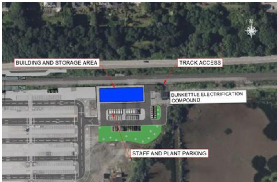
Figure 6-6 Electrification Compound – General Layout
