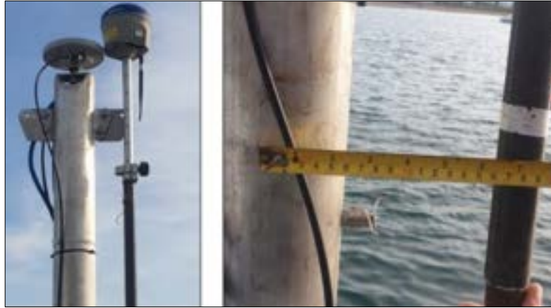
Figure 8: GNSS Rover location (left picture) and offset from primary GNSS antenna and average results (right picture).
