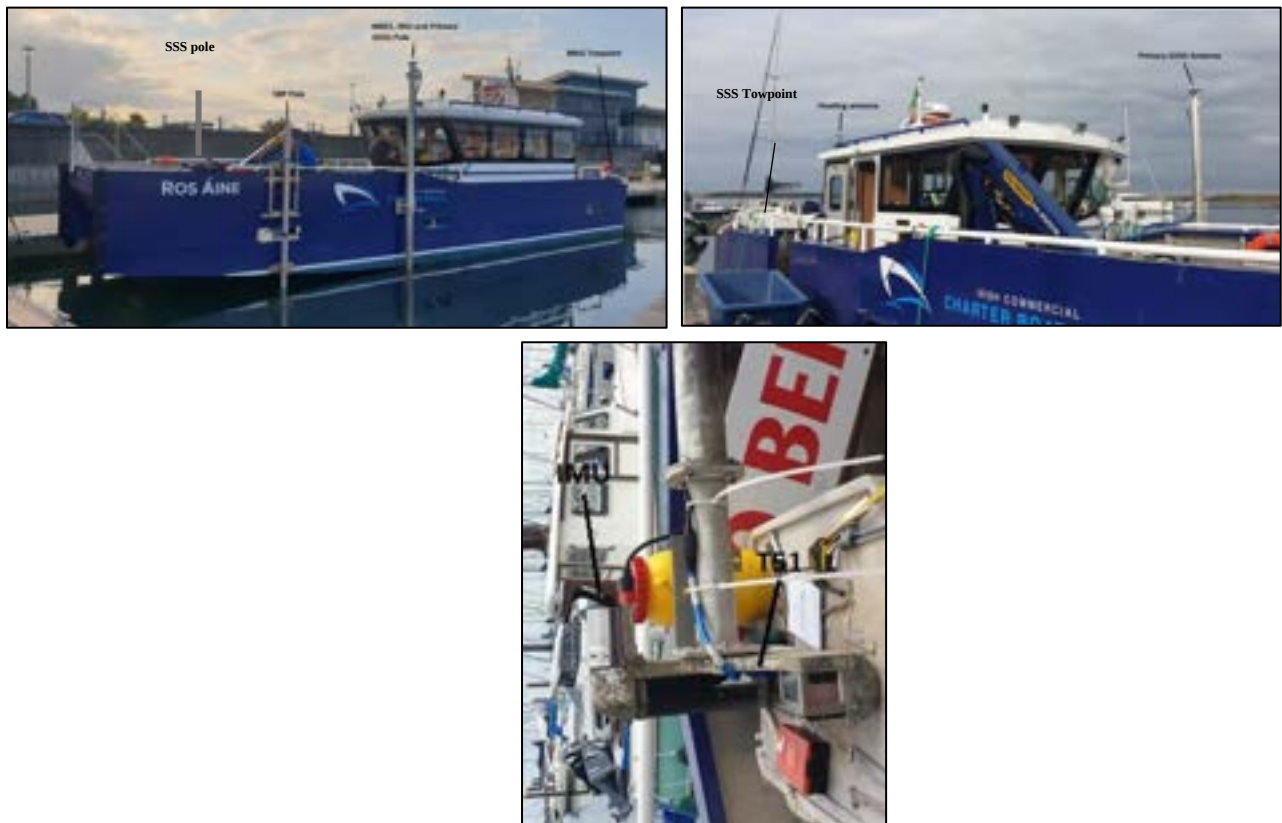
Figure 7: SBP and MBES poles (top left), primary and heading GNSS antennas (top right) and mounting for IMU and MBES (bottom).
