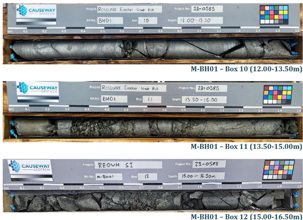
Figure 5-8: Dolerite core recovery from M-BH01.
