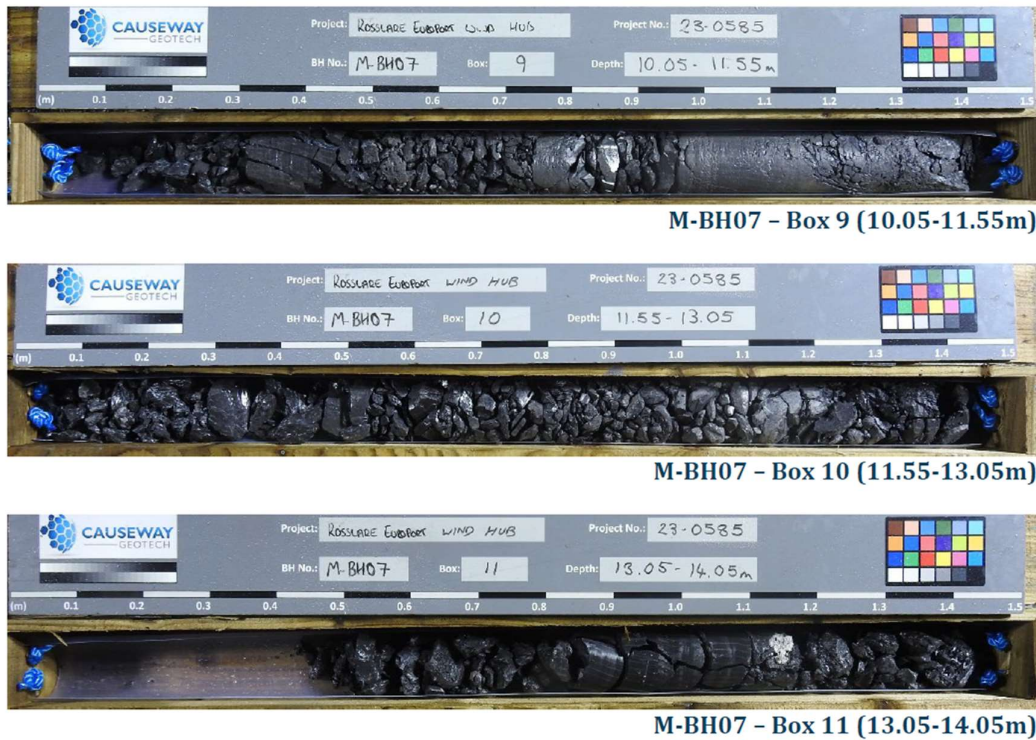
Figure 5-4: Highly fractured and fissile mudstone recovered from M-BH07, illustrating the poor recovery prevalent within the mudstone strata.
