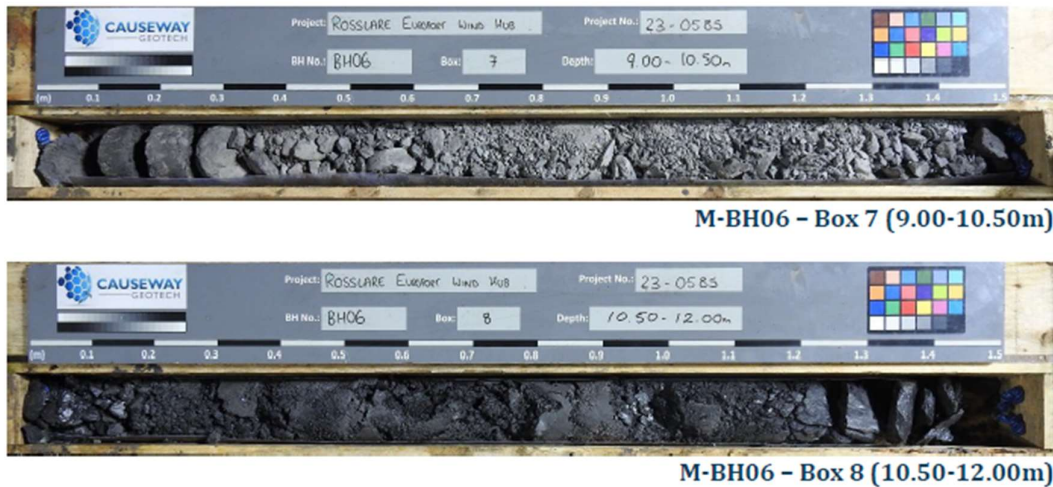
Figure 5-2: Weathered mudstone recovered from M-BH06.
