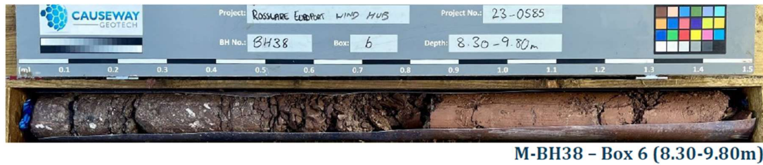
Figure 5-9: Mylonite (possible fault gouge) recovery from M-BH38.
