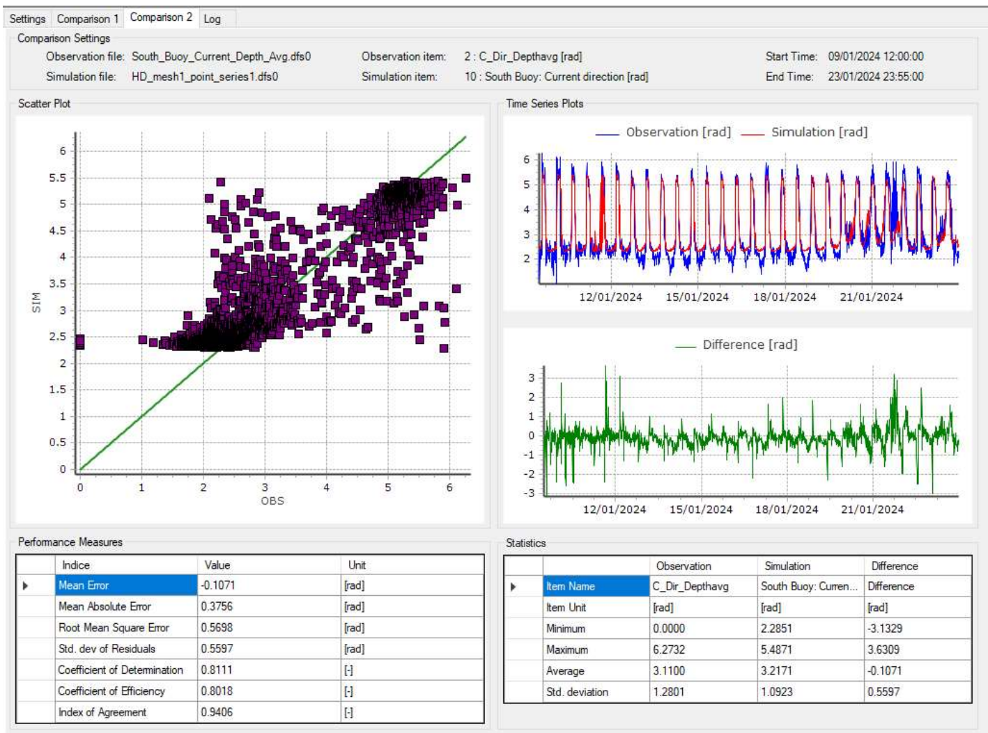
Figure 8-33: Comparison of Measured Depth-Average Current Direction (WB002) and Simulated Depth-Average Current Direction (Source: MIKE21 Time Series Comparator)
